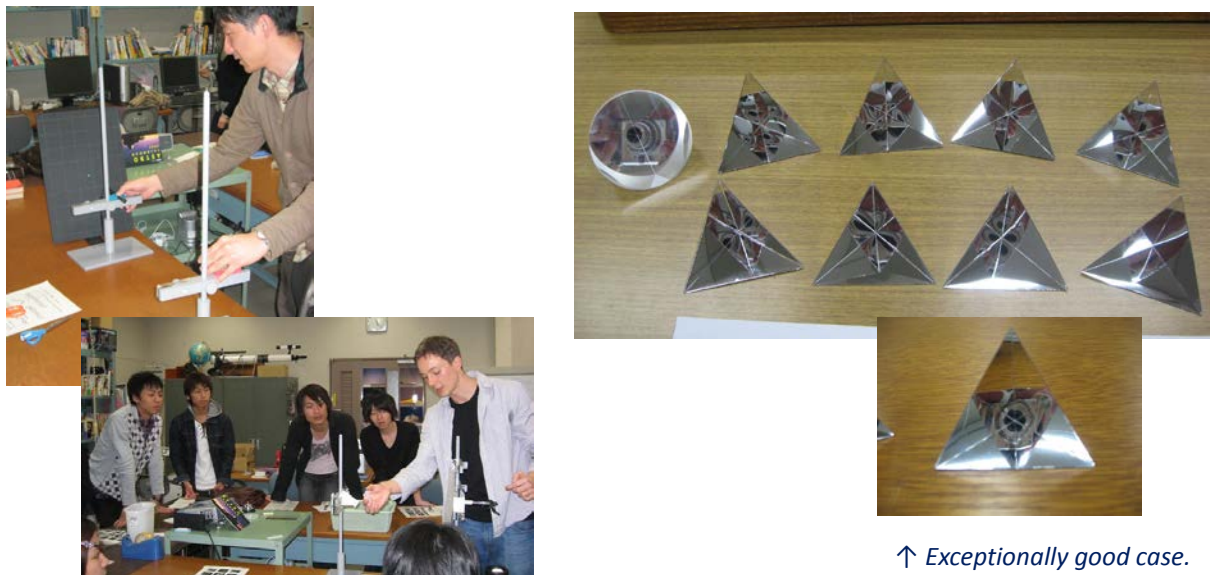
Figure 2. Quality checks of the hand-making corner cube reflectors. Left: pointing a laser beam. Right: taking a photograph.
